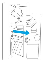
3. Pull the colored tabs away from the assembly, and then pull them up remove the two staple cartridges.
