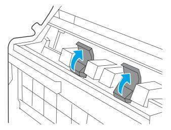
4. Push in the two blue tabs, and then lift up to open the top of the staple cartridge carriage.
