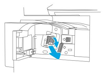
3. Lift two tabs on the staple cartridge, and then lift up to remove the empty staple cartridge from the staple cartridge assembly.
