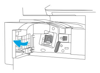
2. Grasp the colored tab on the staple cartridge carriage, and then pull the staple cartridge carriage straight out.
