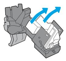
NOTE: Do not discard the staple cartridge carriages. They must be reused with the new staple cartridges.
