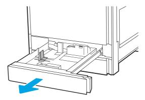
Before loading paper, adjust the paper-width guides by holding down the blue lock/unlock toggle switch on the rear paper-width guide, pinching the blue adjustment latch on the front paper-width guide, and then sliding the guides to the fully open position.
