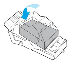
6. Hold the knob to immobilize the staple cartridge assembly, insert the new staple cartridge into the assembly, and then press the colored handle inward until it snaps into place.
