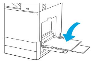
5. Using the adjustment latch, adjust the side guides so that they lightly touch the paper stack, but do not bend it.
