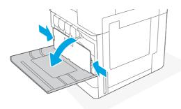
2. Select the **Eject** button from the control panel to eject the cartridge, and then grasp the end of the toner cartridge and pull it straight out of the printer.
