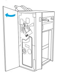
2. Rotate the knob counterclockwise to move the staple cartridge assembly all the way to the front.
