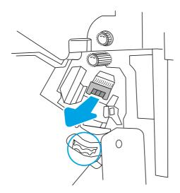
4. Lift two tabs on the staple cartridge, and then lift up to remove the empty staple cartridge from the staple cartridge assembly.
