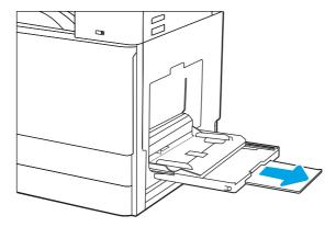
3. Use the adjustment latch to spread the paper guides outward.
