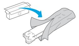
4. Hold both ends of the toner cartridge and rock it to evenly distribute the toner that is inside. And then, remove the seal.
