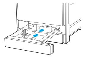
3. Adjust the paper-length guide by pushing in at the bottom of the blue adjustment latch while sliding the guide to the size of the paper being used.
