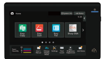
10.1" (diagonally measured) customizable touchscreen display.
